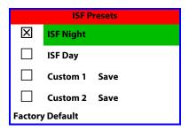
For each input, the Vision 85 lets you save image quality settings as presets that you can recall at a later time. You can create up to four presets per input and resolution. Use the ISF Presets menu to recall saved image presets, or to save image settings in the "Custom 1" or "Custom 2" memory location. The currently-selected preset is indicated by a "\overline{\times}" to its left; in the example shown here, ISF Night is selected.
